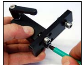
Fig. 3.6.3 TRIXY assembly bracket with support tube
